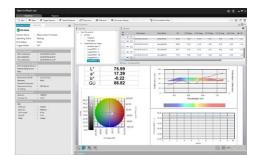
The new Color Data Software SpectraMagic DX enables easy management of data measured with the CM-25cG, and offers a new Instrument Diagnosis function to help ensure continued high instrument performance.
