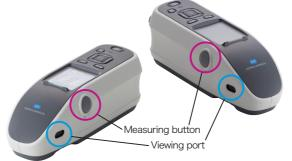
By using a 45°c:0° illumination/viewing system with ringshaped illumination having light sources radially located at certain intervals, the CM-25cG provides stable data while minimizing instrument rotational effects. The system also provides data with high accuracy and repeatability even if there is a small gap between the measurement aperture and the subject.
