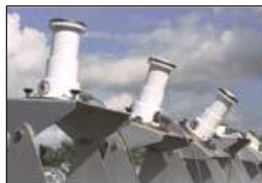
Q-Lab Weathering Research Service offers both typical direct exposure testing and special services. Shown above are AIM (automotive interior materials) boxes, designed to simulate the environment inside an automobile.
