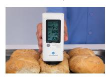
Using the PC application stored in the BC-10 Plus, you can set the instrument to store data internally (Memory capacity: 1000 data), transfer stored data to the PC, or take measurements from the PC.
